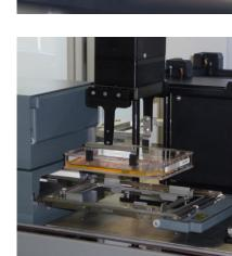
The cell culture system supports all types of automation friendly cell culture flasks which can be compared with standard T75 flasks - Greiner AutoFlask $^{\text{TM}}$ , Corning RoboFlask $^{\text{TM}}$  and BD Falcon Automated cell culture flask. In addition, all types of multiwell culture plates and microtiter plate format labware are supported by the system and it's integrated devices.
